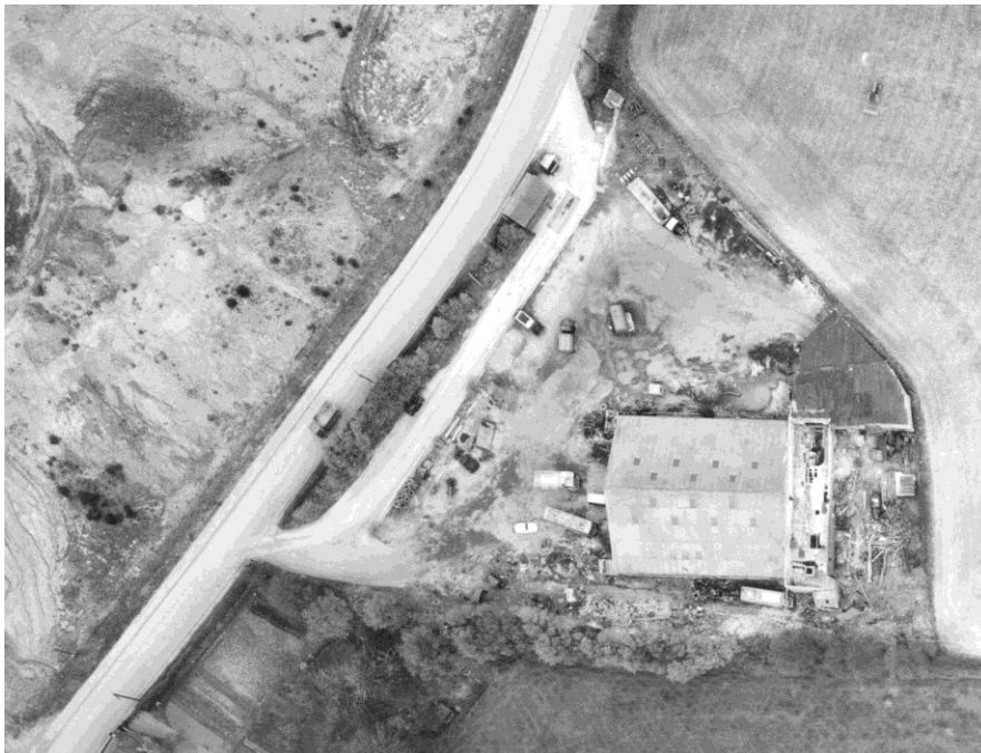
Figure 3. The site in 1961. At this time, it was being used as a depot by the Clay Colliery Company in association with the Opencast site on the opposite side of the road. The kilns have been demolished and the clay preparation area is unroofed. The main production building is being used as a garage. A weighbridge has been constructed at the north end of the site adjacent to the main road.
