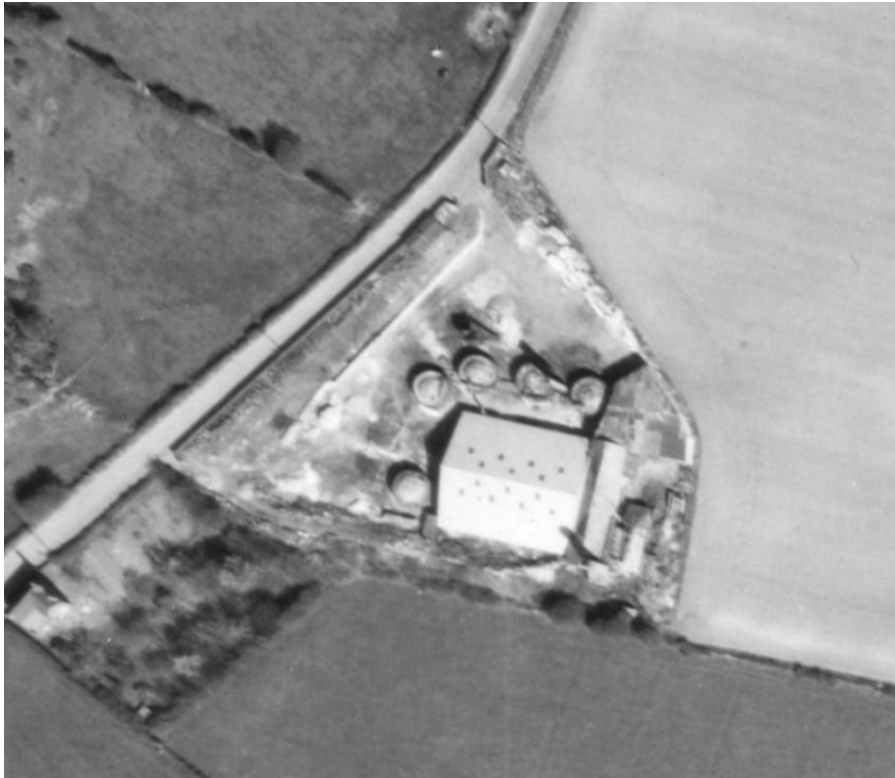
Figure 2 The site in 1953. Production had moved to Lightmoor but only one kiln has been demolished the site appears to be intact. Since 1946 the main production building has been re-roofed and incorporates skylights. (National Archives RAF 82_769_v_005)
