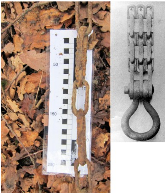
Figure 8. Left: Remains of winding chain used as fencing. Right: Example of the triple-linked winding chain as listed in the sale documents and used for fencing. (IGMT)
