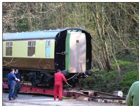
Rolling the carriage off the trailer and on to a temporary stretch of track
