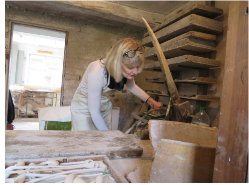
Volunteer Linda Hardman demonstrating how to shape a clay pipe the old fashioned way!)
