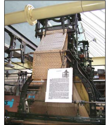
This jacquard loom could weave complex patterns but took several days to thread
