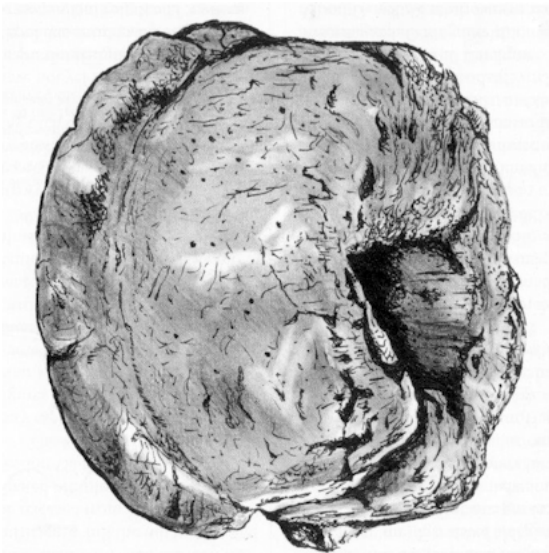
Figure 2. Very early flanged wooden railway wheel, seventeenth or eighteenth century, found at Caughley, Shropshire, 1900-1901. Maximum diameter about 9.5" (24.1 cm). (Sketch by the author)
