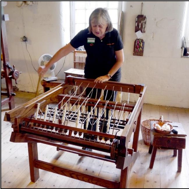
Arkwright's spinning jenny substantially increased the amount of yarn which could be spun by the cottage industry
